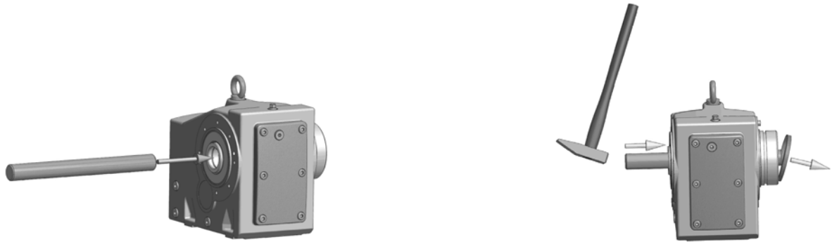
Figure 5: Removing the factory-fitted closing cap
